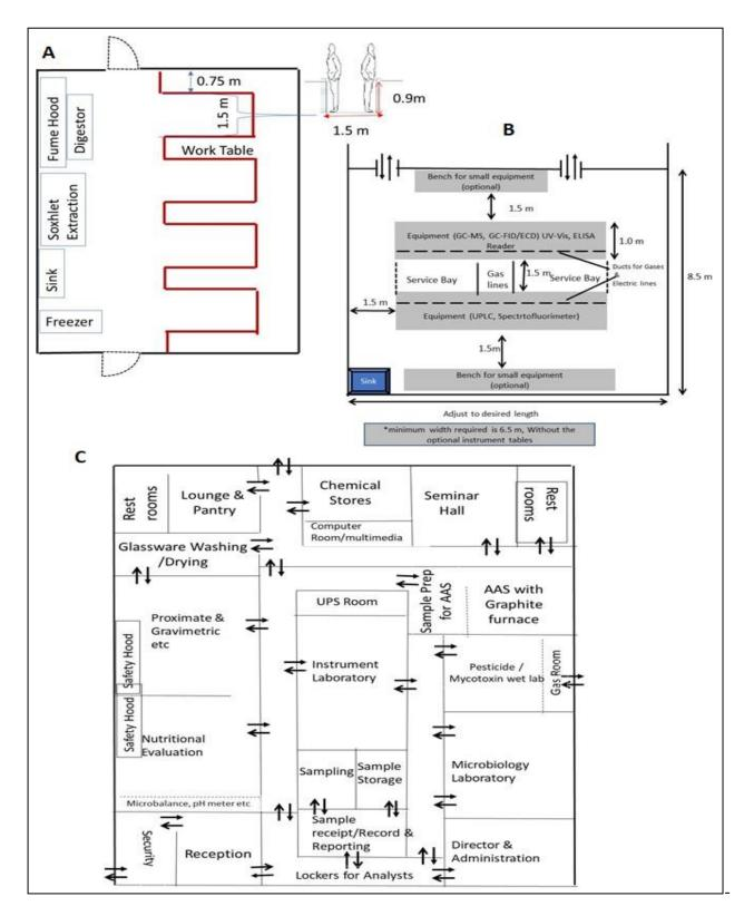
**Figure 5** Schematic layout for A) laboratory for eight analysts B) Instrument room and C) Complete Food Testing Laboratory
