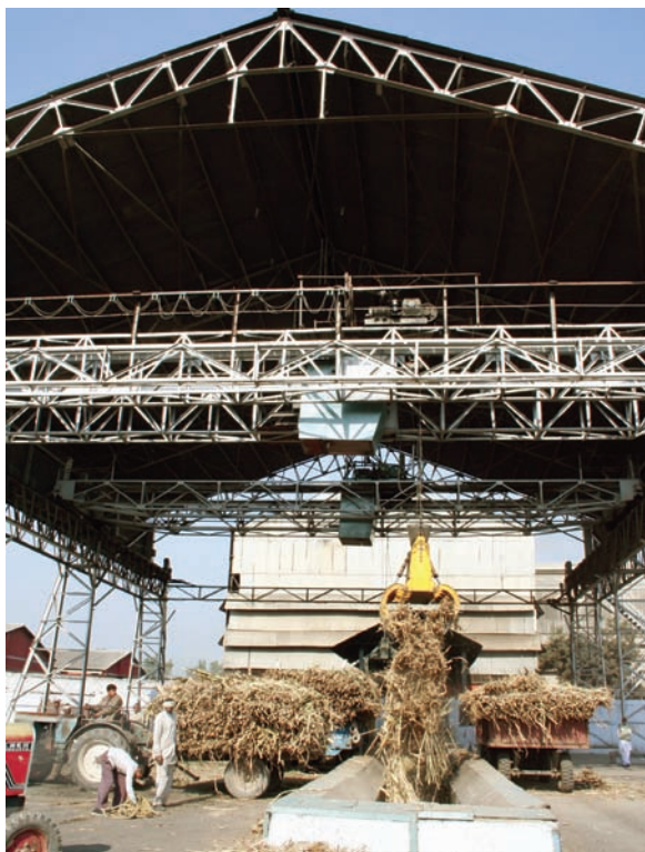
Cane handling operations in a sugar factory.
